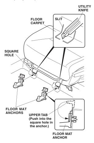
Push the lower tab of the anchor into the square hole concealed under the floor carpet. Pull the upper tab down, and push it into the square hole in the anchor as shown. Repeat on the remaining anchor.
