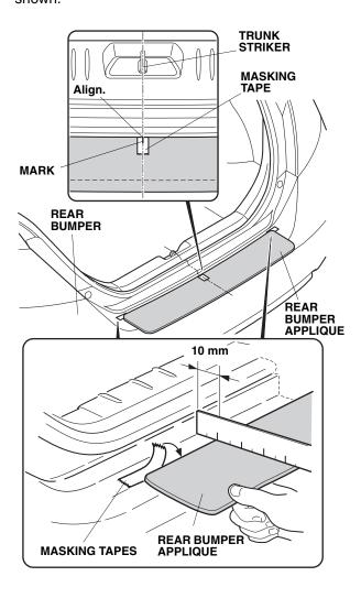
4. Remove the center backing from the rear bumper applique.
