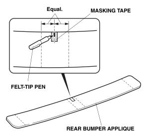
3. Place the rear bumper applique on the rear bumper, then attach masking tapes to the rear bumper as shown.
