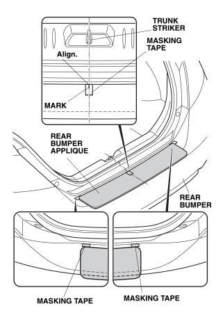
Remove the backing shown. Using the applicator
