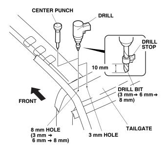
9. Repeat step 8 to drill the tailgate on the right side of the vehicle. Remove any burrs from the edges of the holes using a file, and apply touch-up paint to the edges. Allow the touch-up paint to dry.
