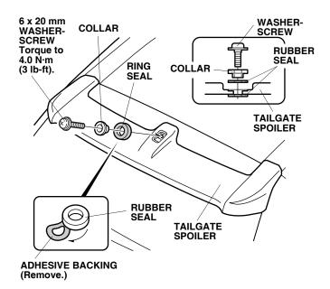
19. Install the collar and 6 x 20 mm washer-screw through the rubber seal and into the tailgate spoiler. Torque the 6 x 20 mm washer-screw to 4.0 N⋅m (3 lb-ft).
