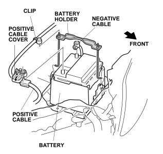
8. Remove the battery cover, battery, and battery tray.
