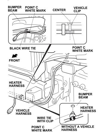
22. Secure the heater harness to the vehicle harness using two black wire ties as shown.
