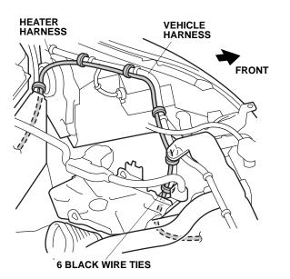
25. Secure the heater harness to the vehicle harness using one white wire tie and five black wire ties in the areas shown.
