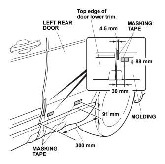
8. Peel back 1-1/2–2 inches of the adhesive backings, and tape them to the front of the rear body side molding. Remove the front and rear adhesive backings.
