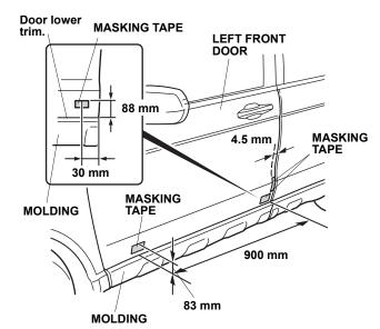
2. Peel back 1-1/2–2 inches of the adhesive backings, and tape them to the front of the body side molding. Remove the front adhesive backing.
