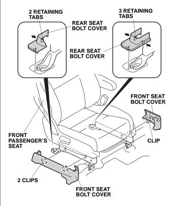
17. Remove the front seat bolt cover from the front passenger's seat (three clips).
