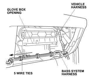
31. Secure the bass system harness to the vehicle harness using five wire ties.
