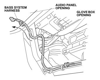
33. Connect the bass system harness 17-pin connector to the vehicle 17-pin connector and secure the connector, to the vehicle harness using one wire tie.
