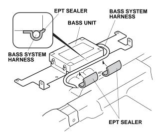
24. Secure the bass system harness to the right bracket using one wire tie with clip.
