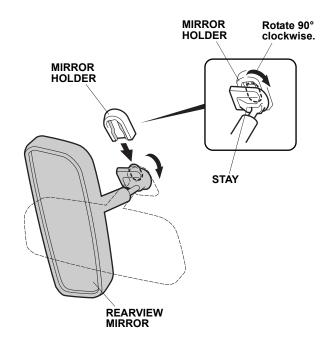
21. Replace the spring. Slide the automatic day/night mirror stay onto the mirror holder, then turn the mirror stay counterclockwise as shown.
