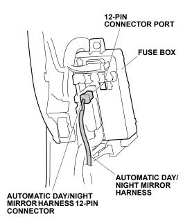
If another accessory connector is using the 12-pin connector, remove the dummy connector from the other 12-pin connector harness and connect the 12-pin connector into the other accessory.
