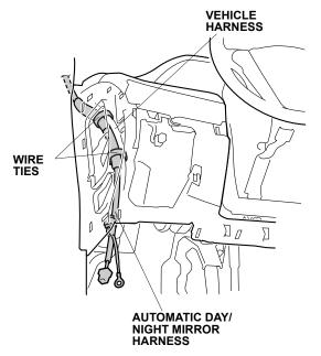
32. Secure the automatic day/night mirror harness to the vehicle harness using two wire ties in the areas shown.
