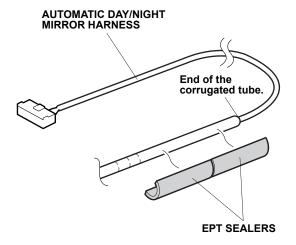
23. Attach a piece of wire to the automatic day/night mirror harness connector, and wrap electrical tape around the wire and the automatic day/night mirror harness. Route the harness to the left front pillar trim opening.
