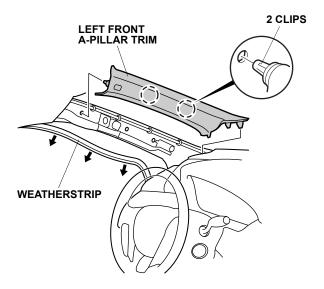
13. Remove and discard the clip from the left front A-pillar trim, and install a new clip (supplied) to the trim.
