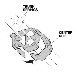
17. With an assistant holding the trunk lid open, remove the old trunk springs from the trunk hinge arms using the trunk spring tool. Wear gloves to protect your hands, and pull the trunk spring tool slowly and carefully towards you.
