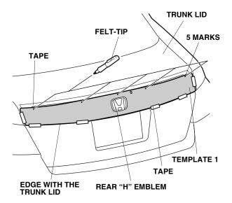
4. Position template 2 (portion A) with the center mark on the tape. Using a felt-tip pen, mark the tape at the notch as shown.
