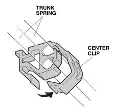
17. With an assistant holding the trunk lid open, remove the old right trunk spring from the trunk hinge arms using the trunk spring tool. Wear gloves to protect your hands, and pull the trunk spring tool slowly and carefully toward you. Do not remove the old left trunk spring.
