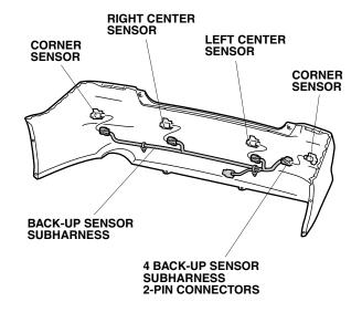
36. Install the two clips from the back-up sensor subharness into the holes of the left center sensor clip and the right center sensor clip.
