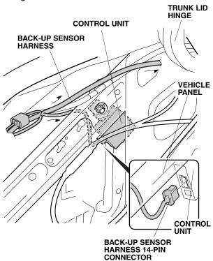
16. Secure the back-up harness to the vehicle harness with two wire ties.
