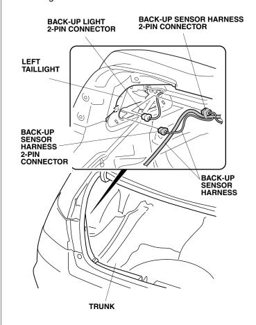
14. Wrap one urethane tape around the back-up sensor harness 2-pin connector, and secure it to the vehicle harness with one wire tie.
