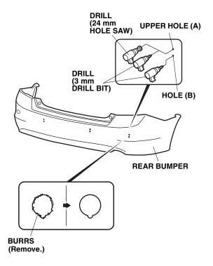
Using a 26 mm hole saw, enlarge the inboard (center sensor) bumper holes by drilling the lower 3 mm holes.
