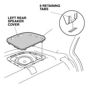
9. Remove the left rear speaker (one bolt and disconnect the vehicle connector).
