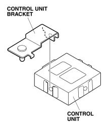
11. By hand, thread the 6 mm flange nut onto the control unit bracket stud. Insert the control unit bracket into the hole in the vehicle panel as shown. Secure the bracket to the vehicle panel.
