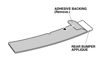
6. Using the spray bottle with protective tape application solution, spray the rear bumper applique.
