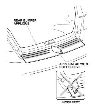
12. Once the flat surface is completely smooth with no bubbles, use the applicator with soft sleeve to apply the rear bumper applique to the rounded rear edge at the center as shown.
