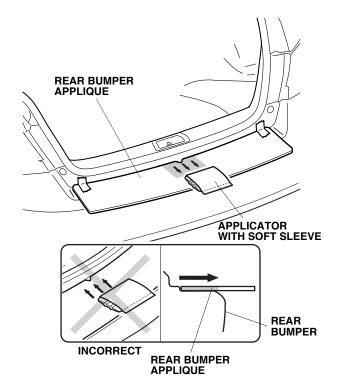
11. Starting from the center and working outward, use the applicator with soft sleeve to smooth the rear bumper applique. Repeat on the right side. Stroke in one direction only.
