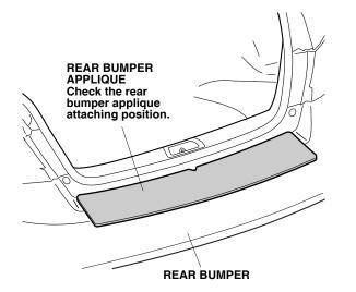
4. Using a spray bottle with protective tape application solution, spray the rear bumper where the rear bumper applique will attach.
