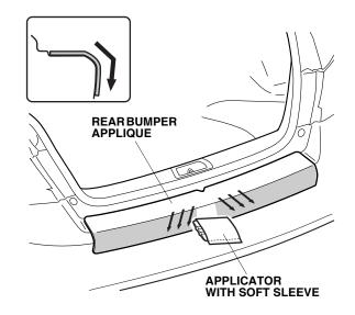
14. Remove the protective film from the top rear bumper applique. Slowly pull the protective film back as you go; do not pull it upward.
