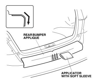
13. Use the applicator with soft sleeve to apply the rear bumper applique to the rounded rear edge on the left side as shown. Start in the middle and work outward. Repeat on the right side.
