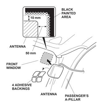
16. Route the antenna harness down the passenger's A-pillar along the vehicle harness, secure the antenna harness to the vehicle harness with three wire ties in areas shown.
