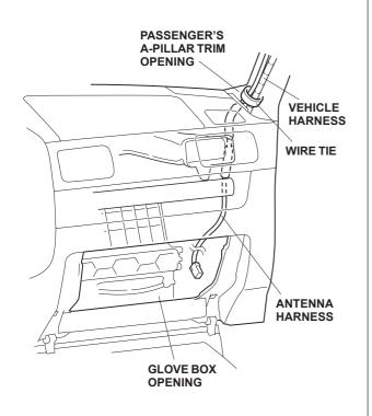
20. Inside the glove box opening, route the antenna harness along the vehicle harness and towards the driver's side of the vehicle. Secure the antenna harness to the vehicle harness with three wire ties in areas shown.
