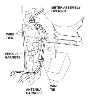
24. Route the antenna harness as shown and temporarily secure it to the vehicle harness using four wire ties.
