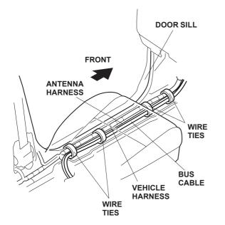
35. Route the bus cable and antenna harness to the top of the car and secure it to the vehicle harness using four wire ties.
