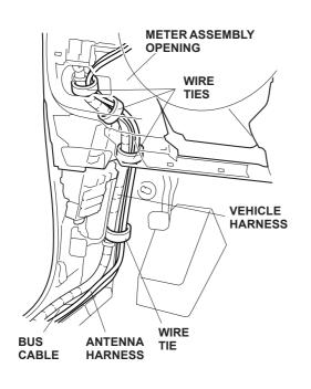
36. Route the bus cable as shown. Secure the bus cable and antenna harness to the vehicle harness using two wire ties as shown.
