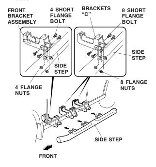
5. Adjust the location of the left side step so that even clearance is obtained between the side step and body, then tighten the long flange bolts you installed in step 3. Torque the long flange bolts to 27 N·m (20 lb-ft)
