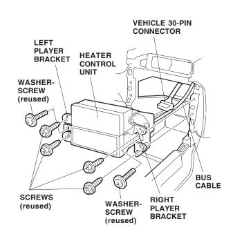
22. Connect the vehicle connectors to the heater control unit, and reinstall the heater control unit using the four screws that you removed in step 10. Go to step 29.
