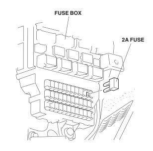
27. Attach the 2A fuse label to the No. 33 slot on the fuse box cover.
