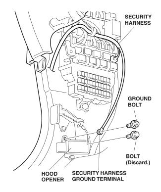
12. Remove and discard the upper hood opener bolt. Get the ground bolt from the kit, and install the ground bolt with the security harness ground terminal to secure the upper hood opener. 13. Secure the ground terminal from the security harness to the vehicle harness with two wire ties.
