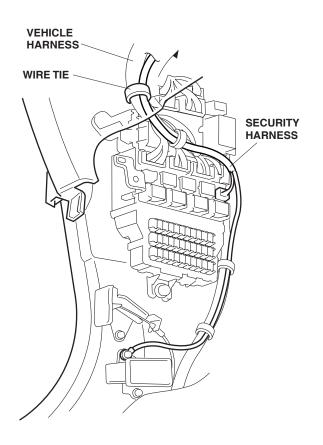
15. Continue routing the security harness along the vehicle frame, and secure it with one wire tie. Wrap one wire tie with clip around the security harness and attach the wire tie with clip to the hole in the vehicle frame.
