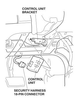
18. Plug the security harness 18-pin connector into the control unit.
