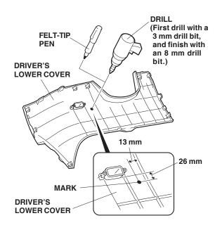
20. While wearing eye protection, drill an 8 mm hole through the marked location. First drill with a 3 mm drill bit, then finish with an 8 mm drill bit. Remove any burrs.
