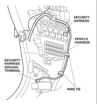
14. Route the security harness up along the vehicle harness, and secure it to the vehicle harness with one wire tie.
