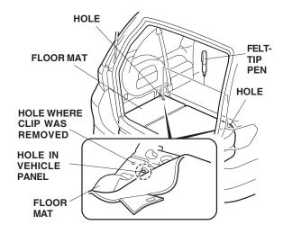
Reinstall the floor mat with the two clips you removed.  Install a stud screw on each anchor. Push the stud screws through the mat at the marks you made in step 3, and secure them to the vehicle panel.
