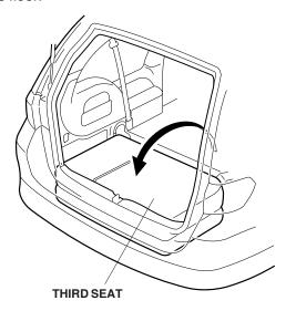
2. On each side, turn over the floor mat, and release the clip from the floor panel. Remove the clips from the resin plates on the floor mat.
