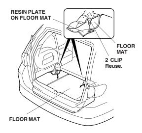
3. Turn over the floor mat. Locate the holes in the vehicle panel shown, then return the floor mat. Using a felt-tip pen, mark the floor mat at the positions of the holes.
