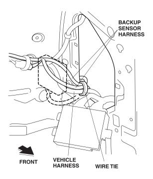
25. If not equipped with a vehicle harness, connect the backup sensor harness to the buzzer and secure the clip on the backup sensor harness to the vehicle panel.
