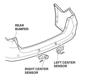
41. From the inside of the rear bumper, insert the right center sensor clip (black) and left center sensor clip (white) to the right center sensor and left center sensor.
