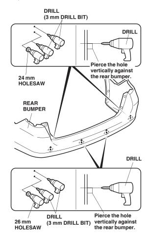
39. While wearing eye protection, drill 3 mm holes at the four pierced marks on the center of the rear bumper from the outside. Widen the two lower holes with a 26 mm holesaw as shown. Remove any burrs.
