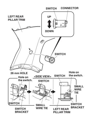
33. Secure the switch bracket to the switch with a small wire tie.
