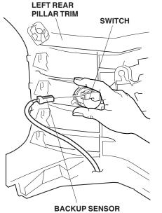
BACKUP SENSOR HARNESS 3-PIN CONNECTOR 7507060B 35. For the left rear pillar trim, insert the clip matching the upper tab and install the trim.
