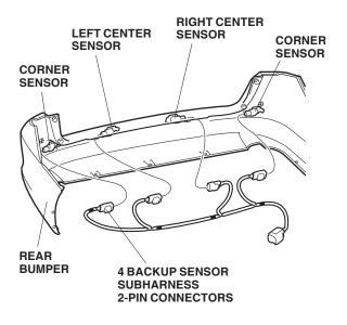
45. Secure the backup sensor subharness connector at the green tape with four wire ties.
