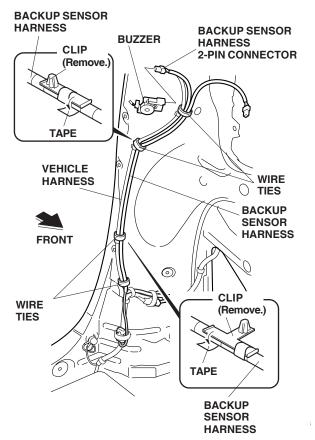
28. Secure the backup sensor harness to the vehicle panel with four wire ties.
