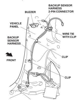
26. Install a wire tie with clip to the backup sensor harness, and secure the clip to the vehicle panel.
