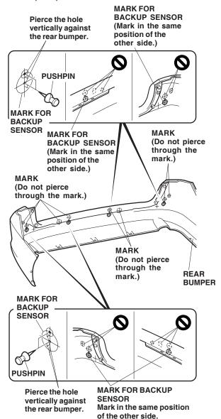
38. While wearing eye protection, drill 3 mm holes at the four pierced marks on the corner of the rear bumper from the outside. Widen the two lower holes with a 24 mm holesaw as shown. Remove any burrs.
