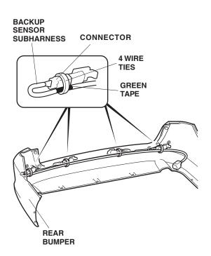
46. Using isopropyl alcohol on a shop towel, throughly clean the area where the harness tapes will attach. Secure the backup sensor subharness to the rear bumper with three harness tapes.
