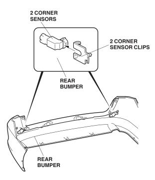
44. Connect the four backup sensor subharness 2-pin connectors to the right center sensor, left center sensor, and two corner sensors.
