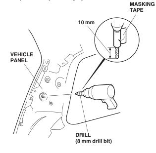
15. Install the blind nut into the 8 mm hole you drilled in step 14. Attach the buzzer to the vehicle panel using the 4 x 14 mm washer-screw. If equipped with a vehicle harness, disengage the vehicle clip from the vehicle panel. Remove the tape and the vehicle clip. Attach the harness clip to the vehicle harness with the tape as shown. Secure the buzzer to the vehicle clip before installing it to the vehicle panel.
