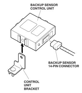
23. Attach the backup sensor control unit to the vehicle panel, and secure the control unit bracket with a 6 mm flange nut.
