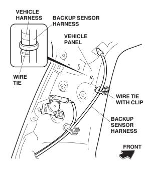
30. Secure the backup sensor 8-pin connector to the vehicle panel.
