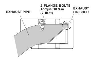
4. Start the engine, and rev it up a few times. Listen for vibration from the exhaust finisher, and adjust if necessary.
