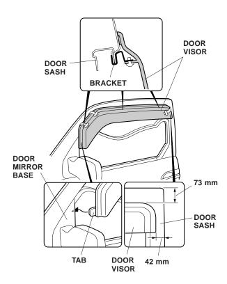
5. Adjust the location of the door visor so that the clearance between the door visor and door sash is 73 mm at the top, and 42 mm at the back. There should be no clearance between the door mirror base and the visor.
