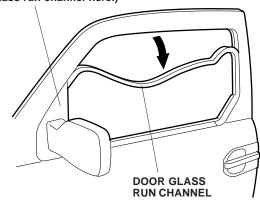
Using isopropyl alcohol on a shop towel, clean the shaded area of the door sash.
