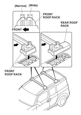
8. If the ends of the right and left roof racks are not aligned, adjust them by loosening the crossbar socket bolts and moving the stays in or out as necessary.
