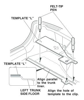
13. Center-punch the marks you made. Lift the trunk liner and check that the center-punched marks you made are centered on the sheet metal rib. While wearing eye protection, drill a 5.5 mm hole through each mark. Start with a 3 mm drill bit and finish with a 5.5 mm drill bit. Remove any burrs, and apply touch-up paint to each hole.
