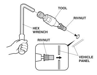
6. While holding the tool with the hex wrench, rotate the 27 mm wrench clockwise and install the rivnut on the vehicle panel.
