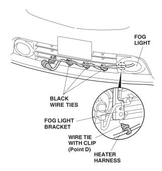
13. Attach the protective cap to the grille, and plug the heater harness connector into the protective cap.
