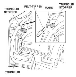
8. Close the trunk lid. Position the template, printed side up, at the left (driver's side) edge of the trunk lid. Align the front hole in the template with the hole in the trunk lid. Using a felt-tip pen, mark the trunk lid as indicated on the template (two marks on the left side).
