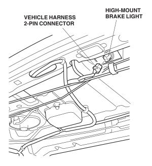
24. Route the vehicle harness 2-pin connector above the trunk springs, and plug it into the spoiler harness 2-pin connector. Secure the 2-pin connector to the vehicle harness with one wire tie in the area shown. Then, go to step 26.
