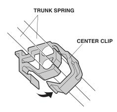
19. With an assistant holding the trunk lid open, remove the old trunk springs from the trunk hinge arms using the special tool. Wear gloves to protect your hands, and pull the special tool slowly and carefully toward you.
