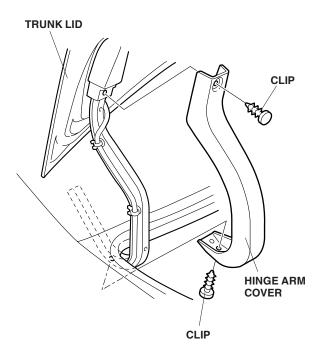
4. If equipped, remove the trunk lid cover (eight clips).
