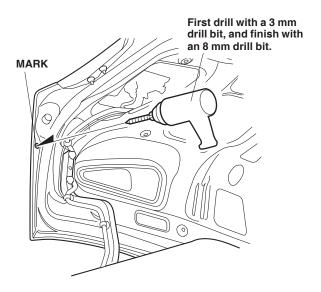
7. Mark the trunk lid stopper with a felt-tip pen, then turn it counterclockwise to remove it. Repeat on the opposite side.
