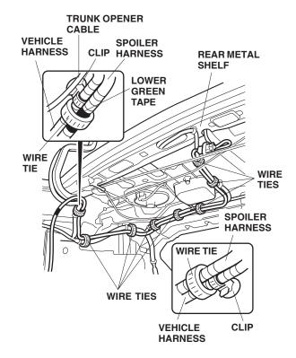
27. Route the spoiler harness alongside the vehicle harness, and secure it with seven wire ties in the area shown.
