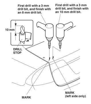
12. Open the trunk lid. Route the harness of the trunk spoiler down through the 10 mm hole you just drilled. Attach the grommet of the trunk spoiler harness to the 10 mm hole.
