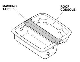
43. Attach template A to the roof console at the indicated position with masking tape.
