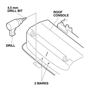
47. Using masking tape, attach the template B to the roof console at the indicated position.
