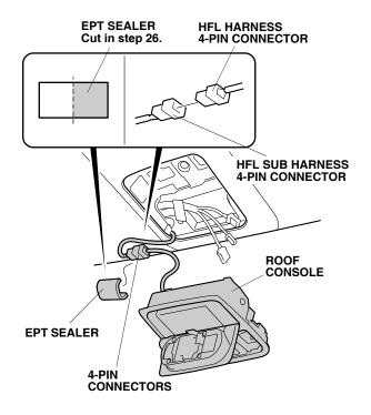
66. Wrap the piece of EPT sealer cut in step 26 around the 4-pin connectors.
