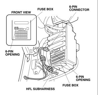
20. If another accessory is already plugged into the 6-pin connector, remove the dummy connector from the 6-pin connector taped to the HFL subharness. Plug the other accessory 6-pin connector into the HFL subharness and plug the HFL subharness into the fuse box. Repeat this step so that these accessories are connected in the following order: (HFL → Automatic Day/Night Mirror → Trailer Hitch).
