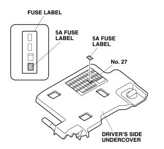
71. Attach the 5A fuse label to the Number 27 slot on the driver's undercover.
