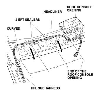
33. Tuck the HFL subharness between the vehicle panel and the headliner. Be careful not to crease the headliner.
