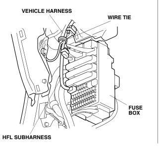
28. Route the HFL subharness along the left A-pillar and secure it to the vehicle harness with four wire ties.
