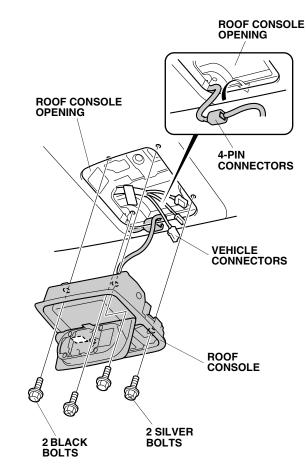
68. Reinstall the roof console.
