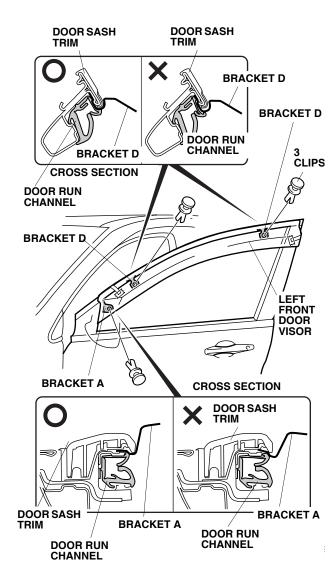
20. Using the palm of your hand, press down on the left front door visor while removing the two adhesive backings. Make sure there is no clearance between the bracket and door sash trim.
