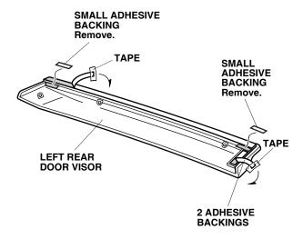
7. Remove the masking tape you attached in step 4.
