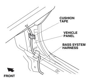
28. Secure the bass system harness to the vehicle harness using one wire tie.
