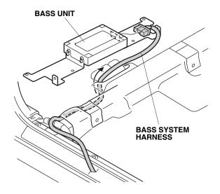
23. Secure the bass system harness to the bass unit using the two EPT sealers.
