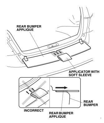
11. Starting from the center and working outward, use the applicator with soft sleeve to smooth the rear bumper applique. Repeat for right side. Stroke in one direction only.
