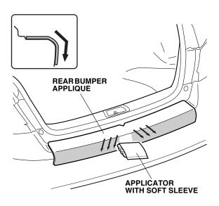
14. Remove the protective film from the top rear bumper applique. Remove the protective film slowly; do not pull up the protective film.
