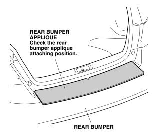
4. Using a spray bottle with 3M protective tape application solution, spray the rear bumper where the rear bumper applique will attach.
