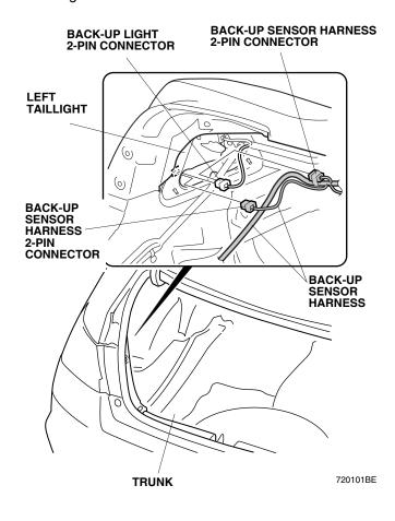
14. Wrap one urethane tape around the back-up sensor harness 2-pin connector, and secure it to the vehicle harness with one wire tie.
