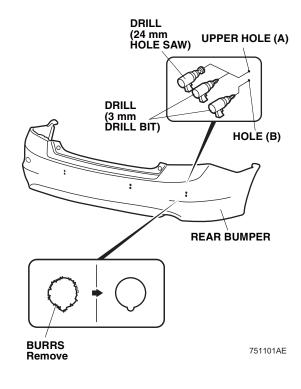
34. Using a 26 mm hole saw, enlarge the inboard (center sensor) bumper holes by drilling the lower 3 mm holes.
