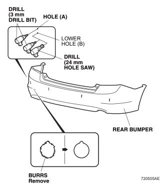
33. Using a 24 mm hole saw, enlarge the outboard (right and left corner sensor) bumper holes. On the driver's side, drill the lower 3 mm hole. On the passenger's side, drill the upper 3 mm hole.
