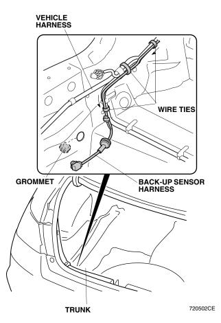
28. Locate and remove the rubber grommet from the rear panel.
