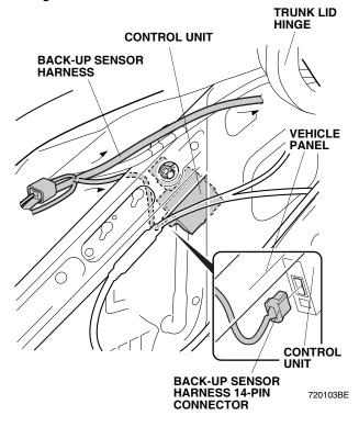
16. Secure the back-up harness to the vehicle harness with two wire ties.
