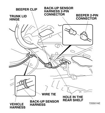
26. Secure the back-up sensor harness to the vehicle harness using one wire tie.
