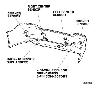
Install the two clips from the back-up sensor subharness into the holes of the left center sensor clip and the right center sensor clip.
