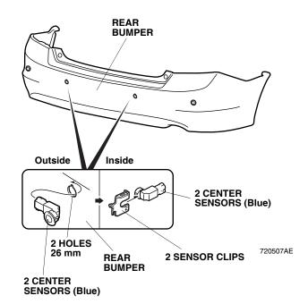
37. Plug in the four back-up sensor subharness 2-pin connectors into the backup sensors.
