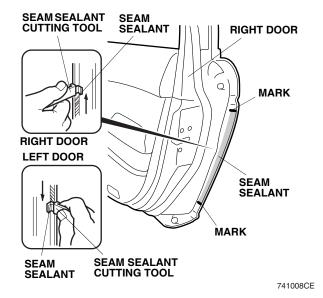
Apply touch-up paint to the cut seam sealant area and let it dry. 7. Position the right door edge guard on the right door edge, and tap it into position with a series of light taps using a rubber mallet.
