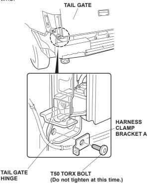
45. Pull the rear camera harness out from the inside of the tailgate, and secure the rear camera harness to the harness clamp bracket A with one small wire tie.
