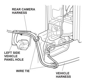
51. Route the rear camera harness out through the bed panel hole, and secure the rear camera harness to the vehicle harness with one wire tie just inside the panel hole.
