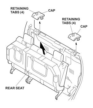
11. Remove the rear trim panel cover (eight clips and two retaining tabs).
