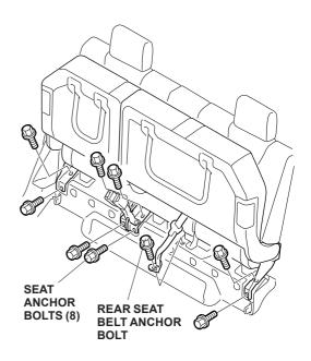
10. Remove the cap from the rear trim panel cover (four retaining tabs for each cover), and remove the rear seat.
