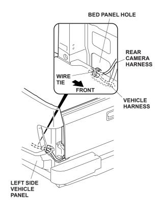
52. Route the rear camera harness along the vehicle harness towards the front of the vehicle, and secure it to the vehicle harness with six wire ties in the areas shown.
