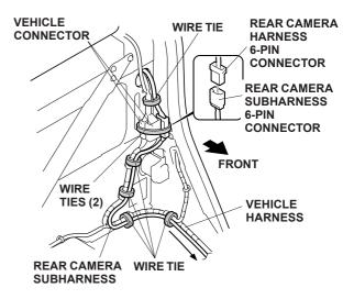
59. Route the rear camera subharness forward along the vehicle harness, and secure the subharness to the vehicle harness with five wire ties.
