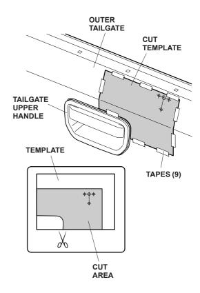
31. Center punch the tailgate at the marks on the template. Remove the template.
