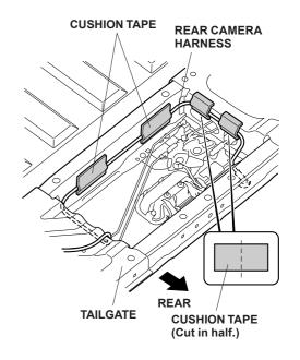
48. Secure the rear camera harness to the tailgate with five wire ties with clip.
