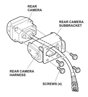
35. Attach a piece of wire to the terminals from the rear camera harness, and tape the wire to the terminals.
