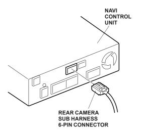
63. Slide the driver's seat back and forth to check that the rear camera subharness is not pulled too tight or is too loose.
