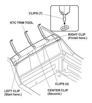
Remove the antenna grommet from the roof, unplug the vehicle connector, and remove the rear roof trim.
