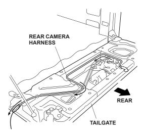
41. Remove the TORX bolt from the tailgate hinge, and attach the harness clamp bracket B to the tailgate using the TORX bolt you just removed. Do not tighten the TORX bolt at this time.
