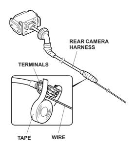
36. Route the rear camera harness through the 10 mm hole in the tailgate, and seat the grommet into the 10 mm hole.
