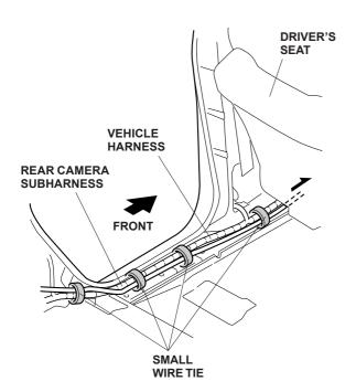
61. Route the rear camera subharness along the vehicle harness and under the floor carpet, then pull the rear camera subharness out from under the floor carpet opening under the driver's seat. Secure the rear camera subharness to the vehicle harness with two wire ties.
