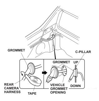
56. Inside the passenger's compartment turn down the rear panel insulator. Pull the rear camera harness out from the hole in the C-pillar, and remove the tape and wire from the rear camera harness.
