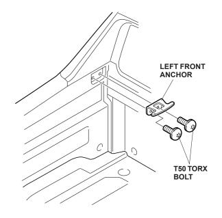
23. Remove the front bed panel (six TORX bolts).
