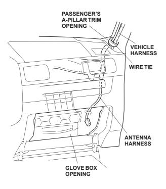
20. Inside the glove box opening, route the antenna harness along the vehicle harness and towards the driver's side of the vehicle. Secure the antenna harness to the vehicle harness with three wire ties in areas shown.
