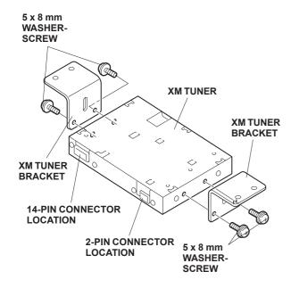
29. Install the XM tuner brackets to the driver's seat panel with four 6 x 16 mm washer-bolts and four 6 mm flange nuts.
