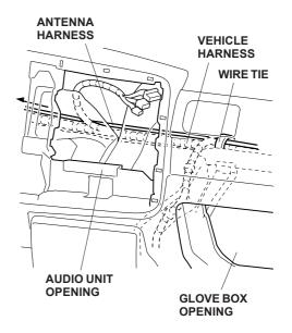
22. Route the antenna harness as shown and temporarily secure it to the vehicle harness using two wire ties.
