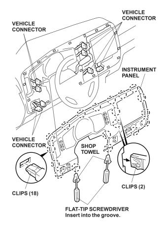
9. Remove the meter assembly (four self-tapping screws, and unplug the three vehicle connectors).
