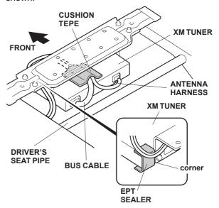
33. Attach the EPT sealer to the corner of the XM tuner as shown.
