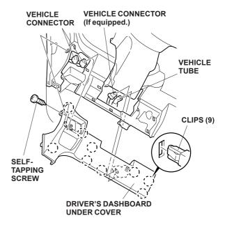
Remove the fuel fill door release handle. Remove the left front door sill trim (three clips and three retaining tabs).
