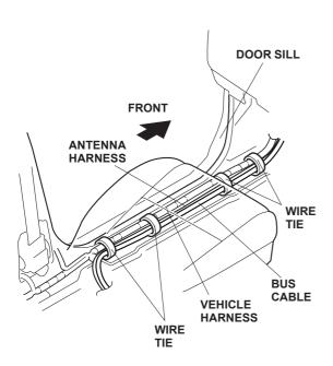
35. Route the BUS cable and antenna harness to the top of the car and secure it to the vehicle harness using four wire ties.
