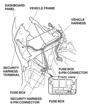
15. Route the security harness 2-pin connector along the vehicle harness, and route the security harness terminal between the vehicle frame and dashboard panel.
