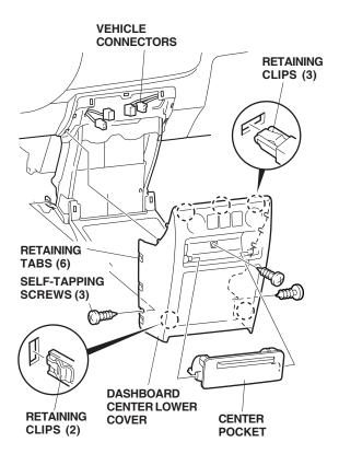
6. Insert a flat-tip screwdriver with a shop towel wrapped around it into the groove of the instrument panel, and release the clips. Pull the instrument panel out toward you to release the eighteen clips, and unplug the vehicle connectors. Remove the instrument panel.
