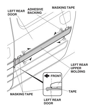
15. Using a hard rubber roller, apply pressure against the molding, and roll from one end to the other.
