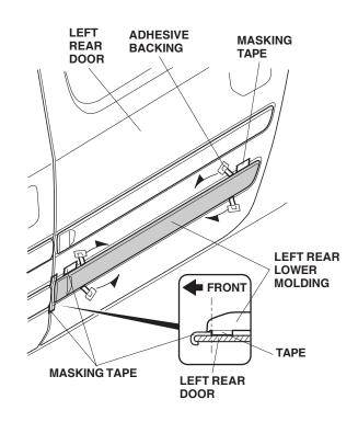
20. Using a hard rubber roller, apply pressure against the molding, and roll from one end to the other.
