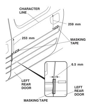
On the inside of the left rear upper molding, attach a strip of masking tape to the ends of the long adhesive backing and peel back 1-1/2 to 2 in.
