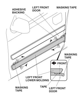
10. Using a hard rubber roller, apply pressure against the molding, and roll from one end to the other.
