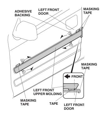
5. Using a hard rubber roller, apply pressure against the molding, and roll from one end to the other.
