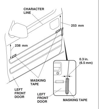
On the inside of the left front upper molding, attach a strip of masking tape to the ends of the long adhesive backing and peel back 1-1/2 to 2 in. (3-5 cm) of the adhesive backing. Tape the ends to the front of the moldings. Remove and discard all other adhesive backings.
