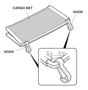
8. Attach the hooks to the anchors in the floor, and attach the loops to the tie-down hooks on the rear side trim panel.
