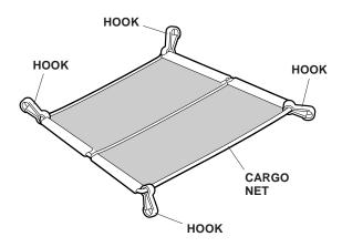
6. Attach the hooks of the cargo net to the front, and to the rear anchors.
