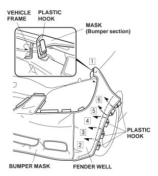
On both sides of the vehicle, attach the five plastic hooks between the fenderwell and the fender in the sequence shown. 8. Insert the four tabs between the headlight and the bumper, and insert the one tab between the radiator cover and the bumper.
