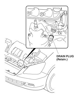
6. Install the engine block heater with the aluminum washer into the hole using a 24 mm socket.
