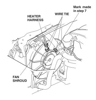
10. Continue routing the heater harness along the vehicle harness and secure the heater harness to the vehicle harness with three wire ties.
