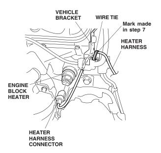
Route the heater harness along the fan shroud and secure the harness with three wire ties.
