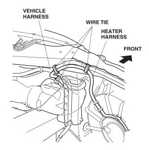
11. Route the heater harness forward along the left headlight, and secure the heater harness to the headlight bracket with one wire tie.
