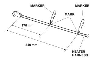
8. Plug the connector end of the heater harness into the engine block heater, then route the heater harness in the direction shown, and secure it to the vehicle bracket with one wire tie at the mark made in step 7.
