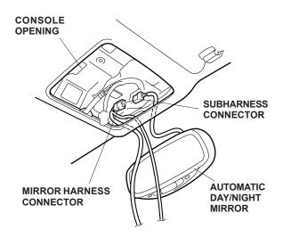
24. Attach the subharness/mirror harness connector to the vehicle panel with one EPT sealer. Position it as far forward as possible.
