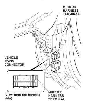
28. Secure the mirror harness to the vehicle harness using three wire ties.
