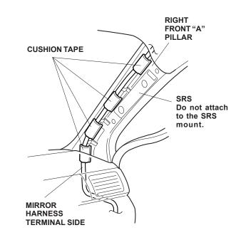
30. Using isopropyl alcohol on a shop towel, clean the headliner area where the mirror harness will attach. Using scissors, cut two EPT sealers in half. Using three halves of EPT sealers, attach the mirror harness to the vehicle panel.
