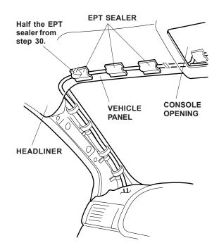
38. Install the wire cover from the mirror to the headliner.
