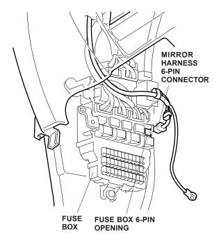
NOTE: If another accessory is already plugged into the 6-pin connector, remove the dummy connector from the 6-pin connector taped to the mirror harness. Unplug the 6-pin connector on the other accessory harness from the fuse box, and plug it into the 6-pin connector taped to the mirror harness. Plug the mirror harness into the fuse box.
