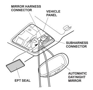
25. Route the terminal from the mirror harness under the headliner toward the right side of the vehicle.
