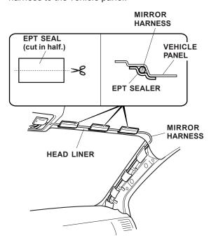
31. Route the ground terminal end of the mirror harness along the headliner and down the left front "A" pillar towards the left fuse box.
