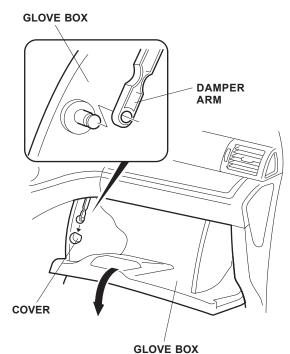
Open the glove box. Remove the two stops by releasing the two retaining tabs for each stop. Remove the glove box (two screws).
