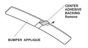
5. Place the applique on the rear bumper at the three 15 mm marks, and center the mark on the masking tape with the latch anchor. Make sure the applique lays flat across the bumper when the marks are lined up. Readjust the applique if necessary, and then erase the marks at each end.
