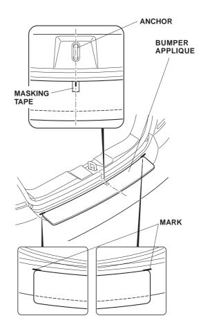
6. Starting from the center, remove about 3 inches of adhesive backing and fold it back. Using the applicator, firmly press the top section of the applique against the bumper. Don't worry about the rear round edge at this time. If you see a bubble, gently peel up that section and work out the bubble. Continue across the bumper 3 inches at a time until finished. Work slowly while keeping pressure against the applique. Adhere the applique to the other side the same way.
