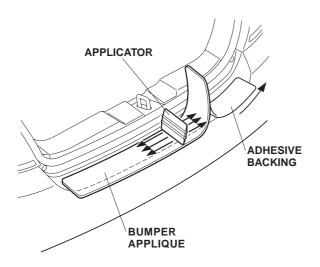
7. Once the top section is finished with no bubbles, use the applicator to adhere the round edge. Start in the middle and work outwards and downwards in small sections. Rub the applicator across and down around the bumper 3 to 4 times to prevent air bubbles. Adhere the applique to the other side the same way.
