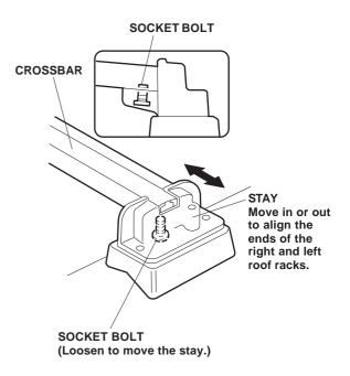
Temporarily tighten the 12 socket bolts and 12 washers.
