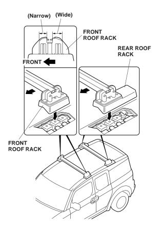
If the ends of the right and left roof racks are not aligned, adjust them by loosening the crossbar socket bolts and moving the stays in or out as necessary.
