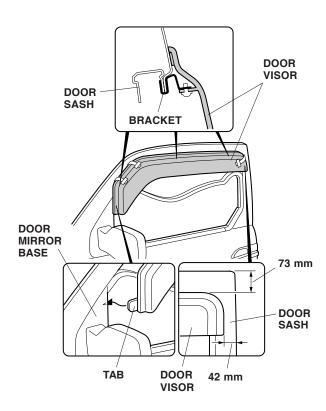
Adjust the location of the door visor so that the clearance between the door visor and door sash is 73 mm at the top, and 42 mm at the back. There should be no clearance between the door mirror base and the visor.
