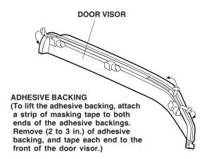
Insert the front tab of the door visor under the door mirror base, and attach the three brackets to the door sash.
