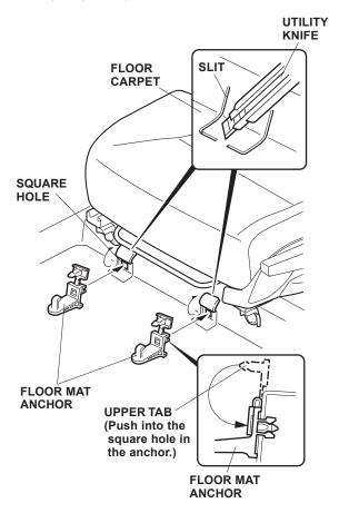
3. Push the lower tab of the anchor into the square hole concealed under the floor carpet. Pull the upper tab down, and push it into the square hole in the anchor as shown. Repeat on the remaining anchor.
