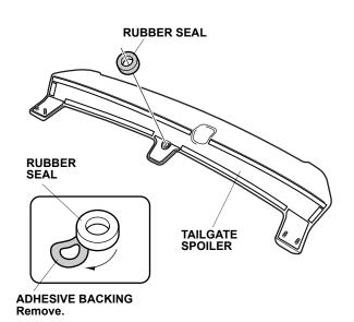
17. Open the tailgate and install the spoiler on the tailgate. Install the four cap nuts to the spoiler studs and torque the cap nuts to 8.8 N·m (6.5 lb.ft).
