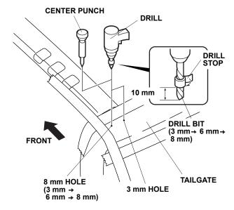
9. Repeat the steps 8 to drill the tailgate on the right side of the vehicle. Remove any burrs from the edges of the holes using a file, and apply touch-up paint to the edges. Allow the touch-up paint to dry.
