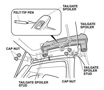
12. Remove the tailgate spoiler, and lightly center-punch the mark you made.
