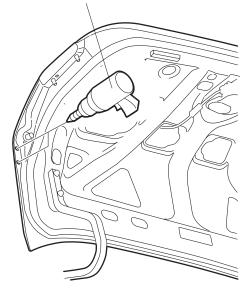
4. Using a paint pen, make a small make across the rubber stopper and trunk lid, then remove the stopper. Repeat on the right side.
