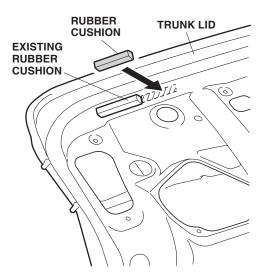
15. Remove the adhesive backing from the rubber cushion, and attach it to the inside panel of the trunk lid next to with the existing rubber cushion. Use the palm of your hand to hold pressure against it for 30 seconds. Repeat on the right side. Then, go to step 21.
