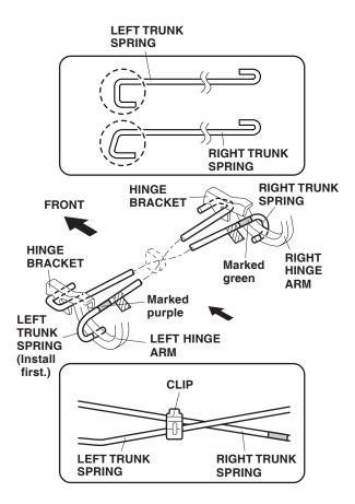
13. Reinstall the center clip on the trunk springs.
