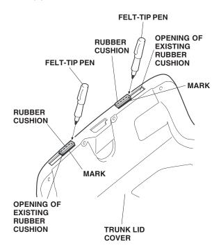
17. Cut out the trunk lid cover with a utility knife along the marks you made in step 17.
