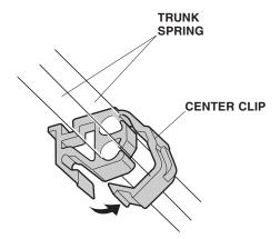
11. With an assistant holding the trunk lid open, remove the old trunk springs from the trunk hinge arms using the special tool. Wear gloves to protect your hands, and pull the special tool slowly and carefully toward you.
