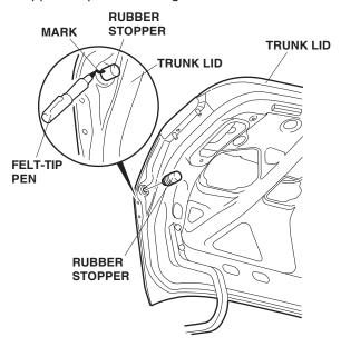
5. Close the trunk lid. Position the template, printed side up, at the left (driver's side) edge of the trunk lid. Align the two outer holes in the template with the two holes in the trunk lid. Using a felt-tip pen, mark the trunk lid as indicated on the template. Remove the template.
