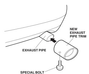
3. With the special bolt on the bottom, slide the exhaust pipe trim onto the exhaust pipe until it bottoms.
