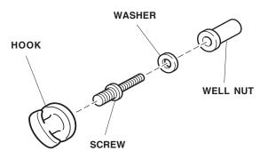
5. Install a well nut/hook assembly into each of the six holes you enlarged, and turn the hook to tighten it in place.
