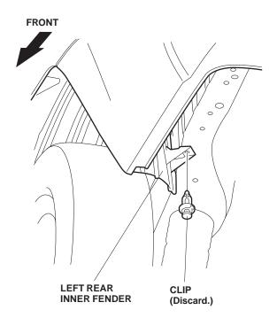
3. Position the left rear splash guard on the left rear inner fender and install the clip from the kit.
