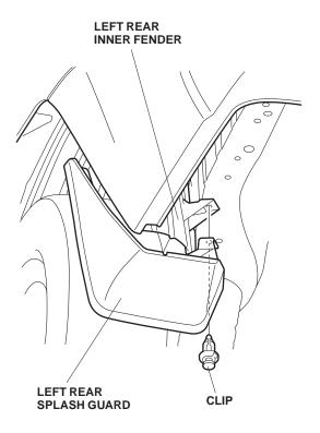
4. While holding the rear splash guard against the bumper, install the splash guard with two self-tapping screws.
