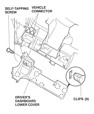
5. Using a tape measure and felt-tip pen, measure and mark the driver's dashboard lower cover.
