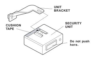
24. Insert the unit bracket into the security unit. Do not push at the connector area.
