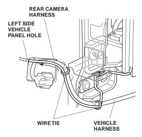
52. Route the rear camera harness out through the bed panel hole, and secure the rear camera harness to the vehicle harness with one wire tie just inside the panel hole.
