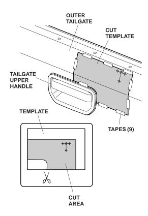
32. Center punch the tailgate at the marks on the template. Remove the template.
