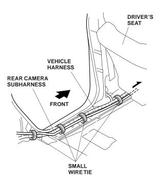
62. Route the rear camera subharness along the vehicle harness and under the floor carpet, then pull the rear camera subharness out from under the floor carpet opening (under the driver's seat). Secure the rear camera subharness to the vehicle harness with two wire ties.
