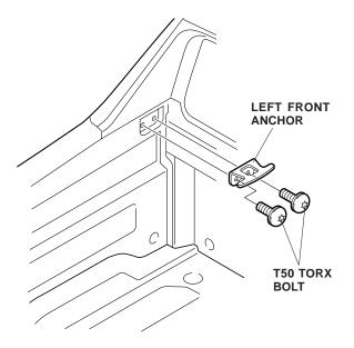
25. Remove the front bed panel (six torx bolts).
