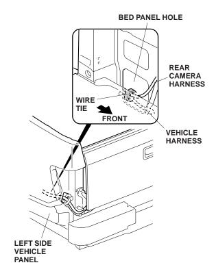
53. Route the rear camera harness along the vehicle harness towards the front of the vehicle, and secure it to the vehicle harness with six wire ties in the areas shown.
