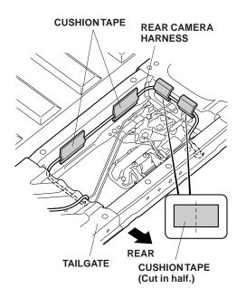
49. Secure the rear camera harness to the tailgate with five wire ties with clip.
