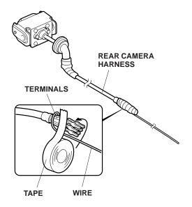
37. Route the rear camera harness through the 10 mm hole in the tailgate, and seat the grommet into the 10 mm hole.
