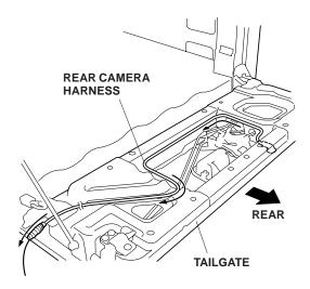
42. Remove the torx bolt from the tailgate hinge, and attach the harness clamp bracket B to the tailgate using the torx bolt you just removed. Do not tighten the torx bolt at this time.
