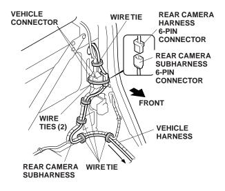
60. Route the rear camera subharness forward along the vehicle harness, and secure the subharness to the vehicle harness with five wire ties.
