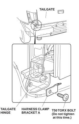
46. Pull the rear camera harness out from the inside of the tailgate, and secure the rear camera harness to the harness clamp bracket A with one small wire tie. Attach the wire tie over the black tape attached to the harness.
