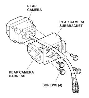
36. Attach a piece of wire to the terminals on the rear camera harness, and tape the wire to the terminals.
