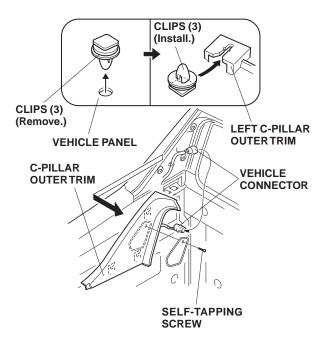
23. Remove the left C-pillar outer trim (slide rearward, and unplug the vehicle connector). Remove the clips from the body, and reinstall the clips to the left C-pillar outer trim.
