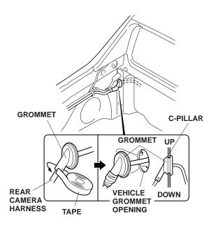
57. Inside the passenger's compartments turn down the rear panel insulator. Pull the rear camera harness out from the hole in the C-pillar, and remove the tape and wire from the rear camera harness.
