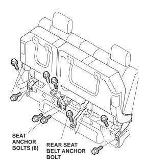
10. Remove the caps from the rear trim panel cover (four retaining tabs for each cover), and remove the rear seat.
