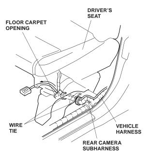
63. Plug the rear camera subharness 6-pin connector into the Navi control unit.
