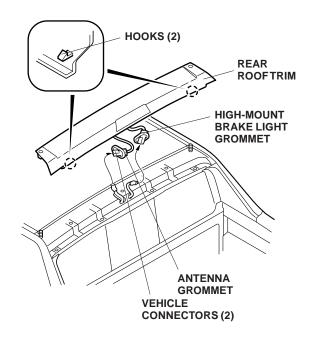
19. Remove and discard the grommets from the roof panel, and install the six oval grommets and one round grommet into the roof panel.
