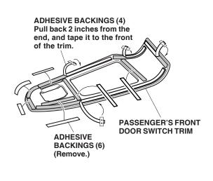
5. Position the passenger's front door switch trim on the existing panel. While holding pressure on the passenger's front door switch trim, carefully remove the adhesive backings from the passenger's front door switch trim. Hold the passenger's front door switch trim firmly against the panel with the palm of your hand, particularly at the edges.
