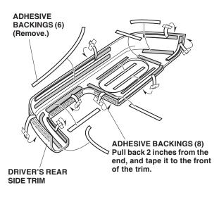
9. Position the driver's rear side trim on the existing panel. While holding pressure on the driver's rear side trim, carefully remove the adhesive backings from the driver's rear side trim. Hold the driver's rear side trim firmly against the panel with the palm of your hand, particularly at the edges. Remove all remaining adhesive backings from the driver's rear side trim.
