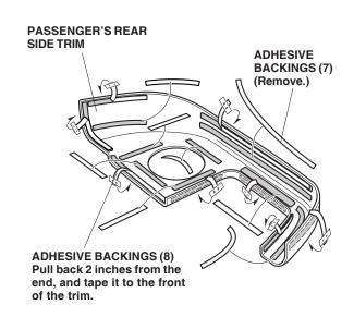
11. Position the passenger's rear side trim on the existing panel. While holding pressure on the passenger's rear side trim, carefully remove the adhesive backings from the passenger's rear side trim. Hold the passenger's rear side trim firmly against the panel with the palm of your hand, particularly at the edges. Remove all remaining adhesive backings from the passenger's rear side trim.
