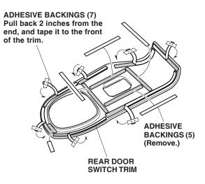
7. Position the rear door switch trim on the existing panel. While holding pressure on the rear door switch trim, carefully remove the adhesive backings from the rear door switch trim. Hold the rear door switch trim firmly against the panel with the palm of your hand, particularly at the edges.
